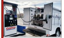
Costco contracts with Crompco, one of the largest gas station testing companies in the U.S. Here's what Crompco says: "From our point of view, Costco has the highest standard in the industry. Costco calibrates all meters every six months and adjusts meters that many retailers would not adjust."
